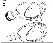
To store the brush nozzle and crevice nozzle, insert brush nozzle vertically into clip then slide crevice nozzle horizontaly until it clips into place
